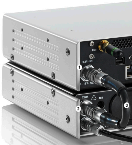
Figure 2-6: Cabling of R&S TSMA with R&S TSMA-BP Battery Pack Unit
